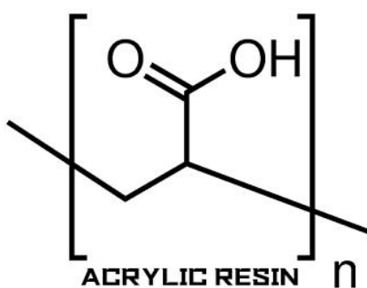
Figure 3 Chemical structural formula of acrylic resin
