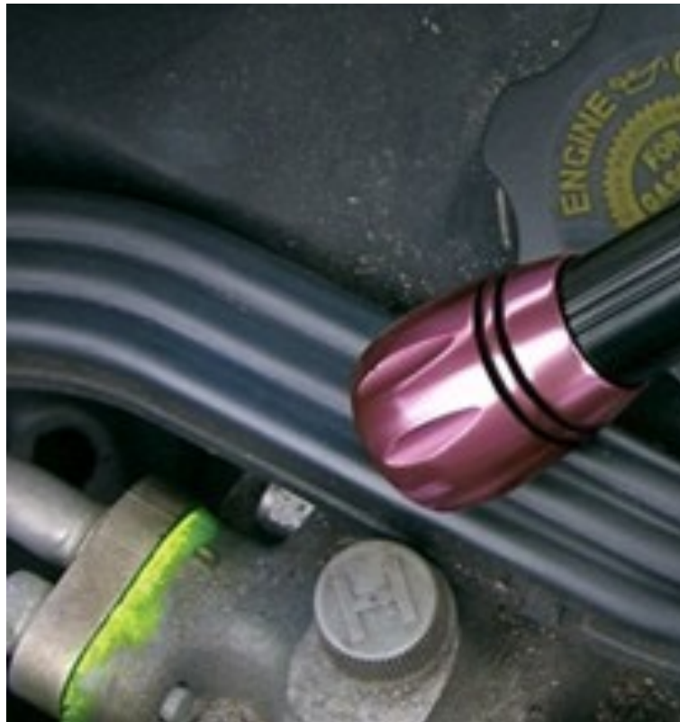
Figure 5 Fluorescence reflection of oil-based fluorescent agent under violet lamp
