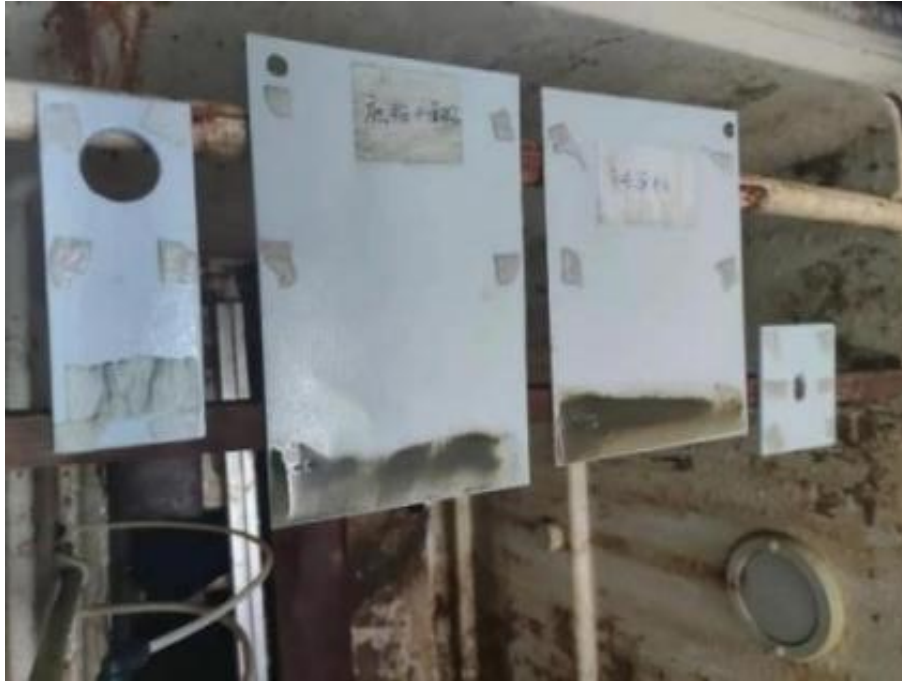
Figure 6 Medium-sized salt spray test for different parts of plates
