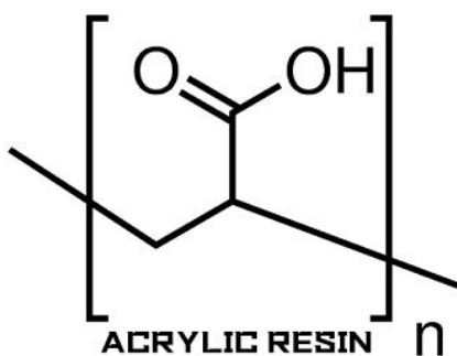
Figure 3 Chemical structural formula of acrylic resin
